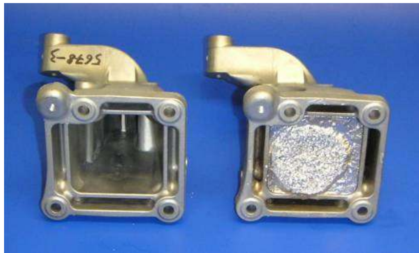
Figure 4.9 SAF filled Engine Bracket
