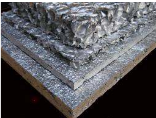
Figure 1.1. Examples of Stabilized Aluminum Foam (SAF) in panel form and as a 3-D casting.
