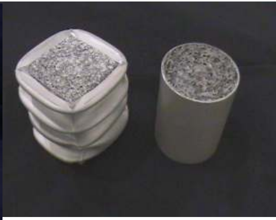
Figure 4.3. Examples of a) a collapsed crashbox and b) a square and round crashbox.
