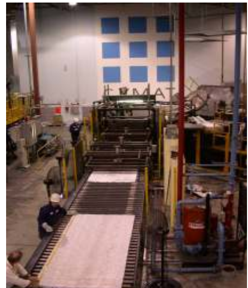
Figure 3.1. The SAF horizontal continuous casting system.
