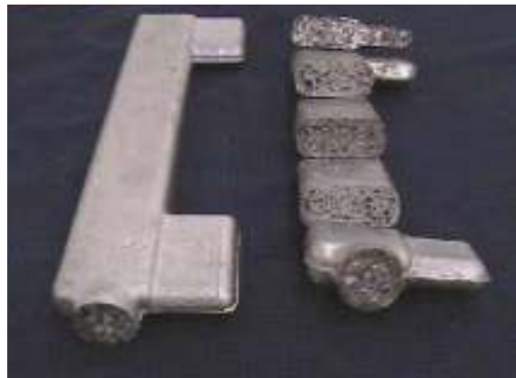
Figure 1.1. Examples of Stabilized Aluminum Foam (SAF) in panel form and as a 3-D casting.
